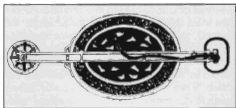
A cutaway drawing of a soft-casing catapult bomb called hekireki kakyū (thunderclap fireball). The lacquered paper casing is filled with gunpowder and pieces of broken porcelain. The fuse is inserted through a bamboo tube. The weight of the object is indicated by the fitting of a wheel and a dragging handle.
